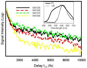
FIG. 2. (Color online)Time evolution of the signal intensity vs delay time  $t_{23}$ with  $t_{12}=0$  for different probe wavelengths. The pump wavelength is 545 nm. The inset shows the photoluminescence (PL) and inverse reflection (1/R) spectra at room temperature.
