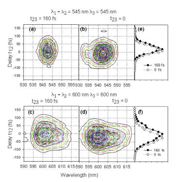
FIG. 1. (Color online) Spectra of three-pulse nonlinear signals vs delay time  $t_{12}$ . The delay  $t_{23}$  is fixed at 160 fs [(a) and (c)] or 0 fs [(b) and (d)]. The wavelengths of the laser pulses are 545 nm [(a) and (b)] and 600 nm [(c) and (d)]. The time evolution of the signal intensity at 545 nm (e) and 600 nm (f) is recorded with a spectral window of 2 nm.
